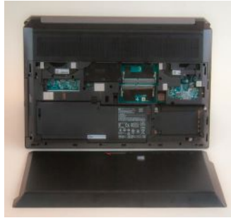
Fig. 2: A removable bottom panel makes it easy to access the interior.
