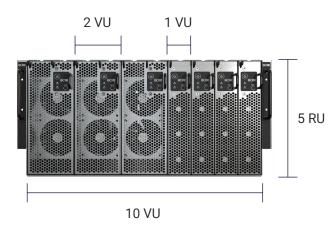
Each enclosure is 5 Rack Units tall and supports 10 VU for system modules. A VU is a "Vertical Unit". System modules come in 1 and 2 VU sizes. Enclosures may be populated heterogeneously with different system modules. Mix and match nodes for any combination of workstation nodes that best suits your workflow.
